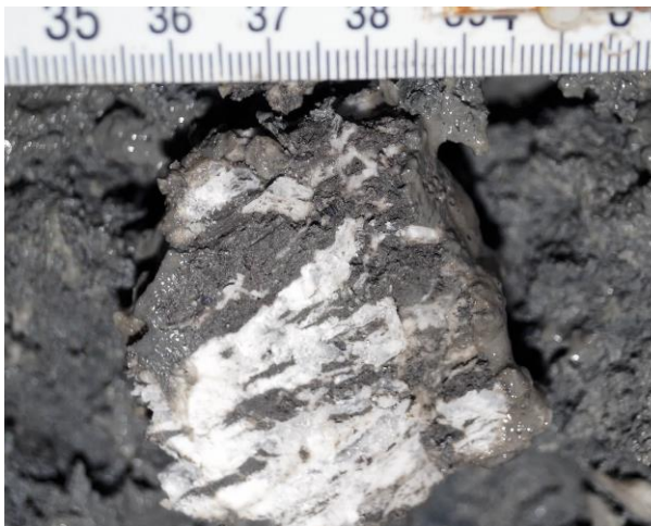
Figure 1: White layers of methane hydrate appear parallel to sediment layering at an active seep within the Lunde pockmark.
