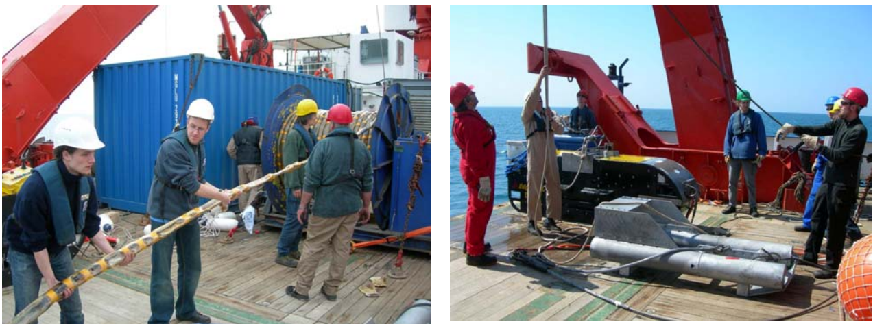
Figure 1: Besides sediment and gas hydrate sampling geophysical tools became more important during the second leg of cruise M72/3. Launching of the 600m-long streamer to perform multichannel seismic investigations (left) and Sidescan Sonar DTS with the depressor in the front just before deployment from the working deck (right image).
