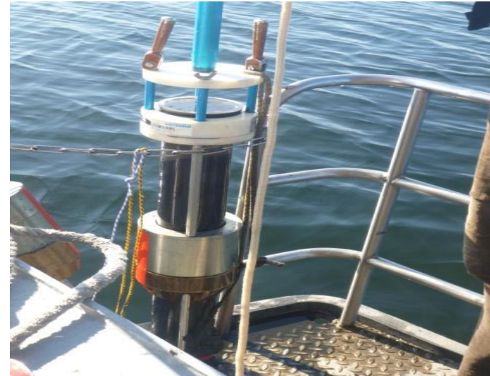
Figure 66: Sampling of a short sediment core at the lake Tegeler See near Berlin.
