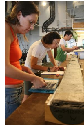
Figure 56: Sediment sampling on board RV Maria S. Merian, Amazon delta. Left: obtaining short sediment cores with a multi-corer. Right: documenting a long sediment core obtained by a gravity corer.
